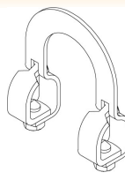
Fig. 015 Large Sway Brace Pipe Attachment
