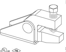
tion: Designed for bracing pipe against sway and seismic disturbances. Universal swivel design allows for attachment at any surface angle combined with concentric loading. Structure attachment fitting designed to use 1" thru 2" SCH 40 pipe, structural steel, and PHD 12 gauge strut channel (1001 & 1201) as sway bracing elements. No bracing member thicker than <sup>3</sup>/<sub>8</sub>" can be used in conjunction with this
